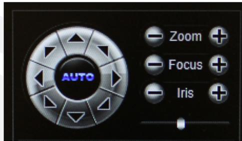
**PTZ control:** 8 directional keys to rotate front-end devices, and AUTO indicates auto-rotation.
